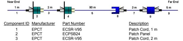
4 **EPCT** KJ32-C6A-FS/ECKJ PANEL-1U 24 Wall Outlet / Patch Panel 5 **EPCT** Port FTP Horizontal Cable 6 C6A S/FTP, 90m **EPCT** Wall Outlet 7 **EPCT** ECSR-V95 Patch Cord, 3 m 8 **EPCT** EC8412S-6A / EC8402BS-6A Wall Outlet **EPCT** 9 ECSR-V95 Patch Cord, 5 m
